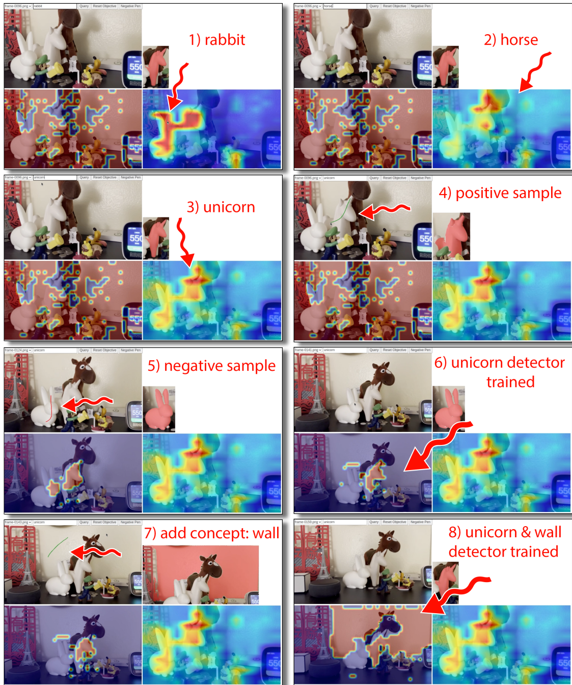
Figure 5.3: Training a segmentation model for arbitrary concepts with in-situ learning. Here we show a new segmentation model for unicorn, a rare concept for existing segmentation models, or even for an arbitrary concept like “unicorn + wall” which can be trained with only a few interactive strokes from the user. Details of the workflow are described in the text.
