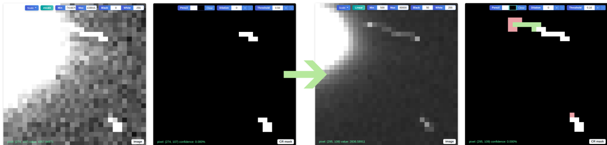
Figure 3.3: When the model or the default threshold does not produce ideal results (left), the user can adjust the HDR image mapping for better visualization, at the same time edit the mask interactively (right). The probability threshold and morphological dilation allow for global mask manipulation, while the pencil tool allows pixel-level mask editing. Pixels that are manually added/deleted by the user are marked in green or red, which will override the global manipulations.
